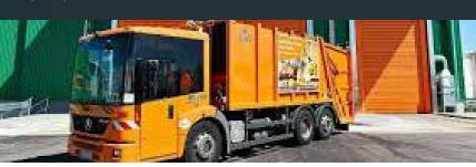
In the German capital, 150 waste management vehicles are fuelled by biogas that is produced by the over 60,000 tonnes of organic wastes that are collected. These vehicles not only provide a reduction in pollution, and two-thirds lower CO2 emissions, but are 50% guieter.11
